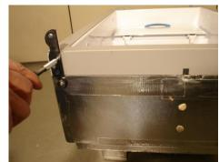
Remove the bottom hinge plate
