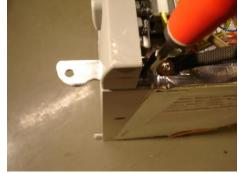
M Place the door on the bottom latch pin
