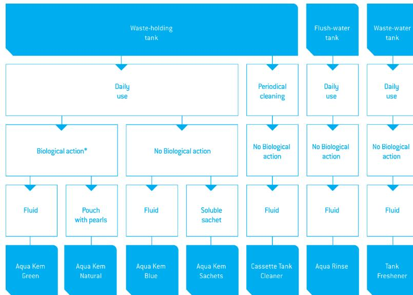
\* Biological action: stimulates micro-organisms to biologically break down the toilet waste in the waste-holding tank. Particularly suitable when emptying the waste-holding tank into septic tanks on camp sites (Test ISO 11734).
